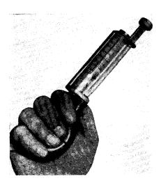
Sulfur Dioxide Detector, available from Mine Safety Appliances Co., is said to be exceptionally accurate yet easy to read and portable. The instrument will detect and determine SO<sub>2</sub> concentrations of 0 to 50 p.p.m. For the determination, the user squeezes the aspirator bulb, then reads the SO<sub>2</sub> concentration directly on a graduated scale
