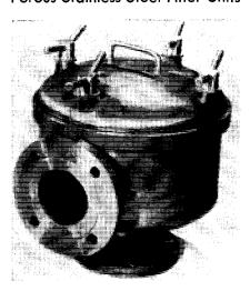
Filter, produced by Micro Metallic Corp. with a filter area of 30 square feet, housed in a stainless steel container 12 inches in diameter and 20 inches long. The compact design of the units permits steam jacketing and sanitary construction. Units with filter areas up to 720 square feet are available PE8
